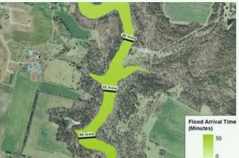
The FIRM for this area in Maricopa County, Arizona shows only a small part of the dam breach inundation area as SFHA. Most of the area is X Zone, where there are no federal requirements for development regulations or for the purchase of flood insurance.
