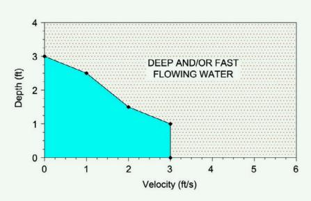
Graphic used to explain Pierce County's Deep and/or Fast Flowing floodway mapping criteria. This graphic illustrates No. 5 on the next page.
