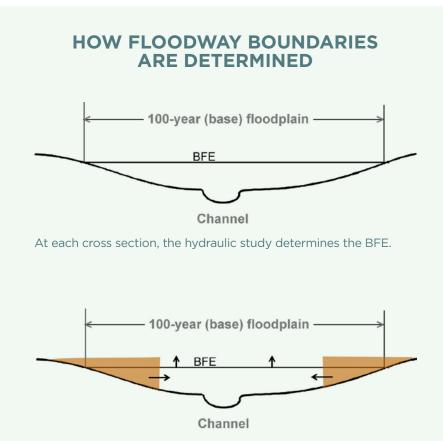
The computer model inserts a virtual obstruction at each edge of the floodplain. This is brought closer to the channel (horizontal arrows). As this happens, the flood level increases (vertical arrows) because there is less area to carry the flow of the base flood.
