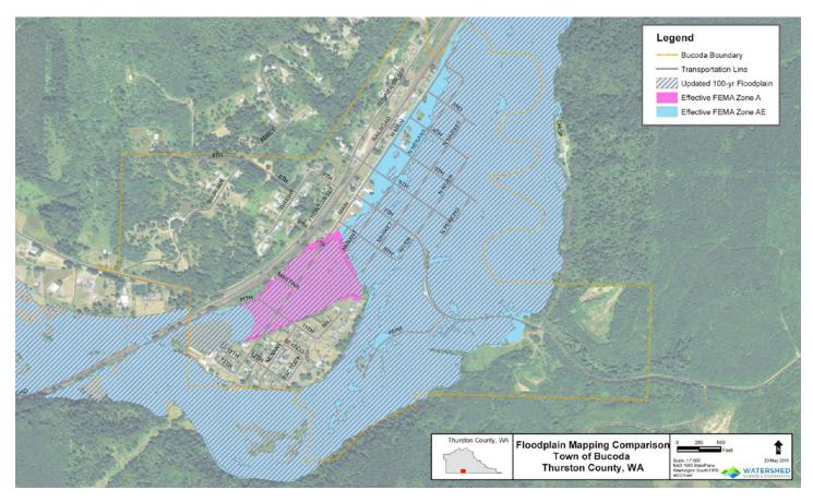
Bucoda's new study provided a BFE for the by-pass (in red). By incorporating all the flows around the island, the new model lowered the BFE and shrank the floodplain upstream of the by-pass. The FIRM's higher BFEs and larger SFHA boundary stay in effect though.
