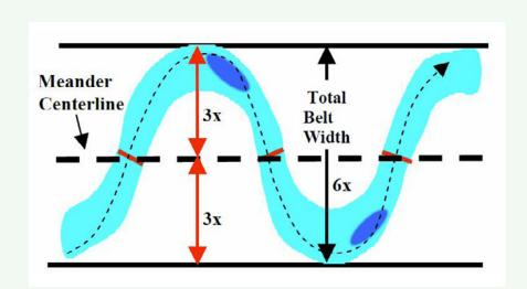
Idealized representation of how a river corridor is mapped: A meander centerline is drawn down the valley and corridor limits are measured out as parallel lines "3 x channel width." Image from pg. 3 in "Defining River Corridors Fact Sheet."
