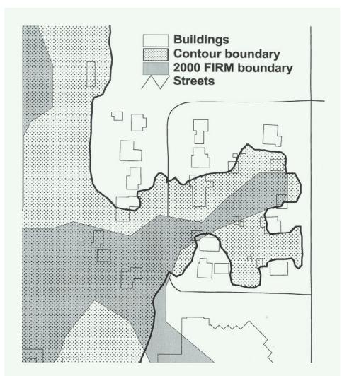
The 2000 FIRM boundary for the SFHA for Gurnee, Illinois was put into a GIS layer. The BFE was plotted on a more accurate village contour map. The differences are significant.
