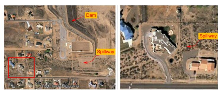
This flood control dam in Albuquerque, New Mexico has an emergency spillway on its south side. The spillway is not mapped as a flood hazard area. Note the area in red, which is enlarged to the right. It shows houses have been built in the path of the spillway's flow. Images from an unpublished paper by Les Bond, 2007.
