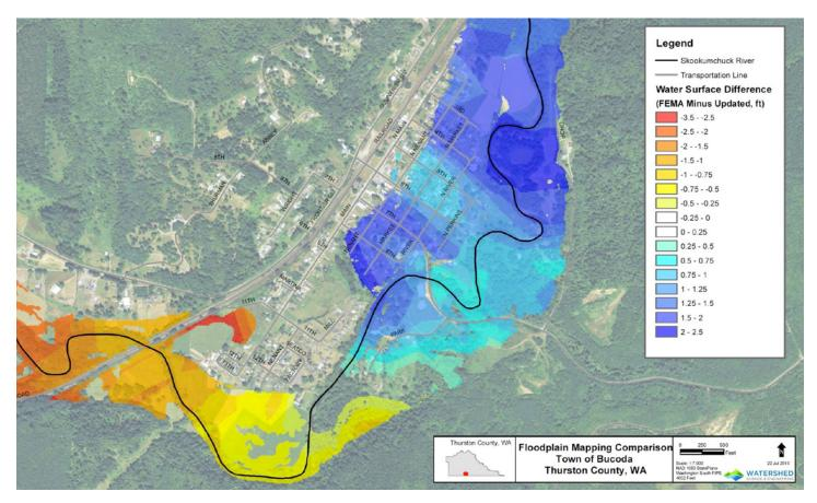
By incorporating more effective flow areas in the model, the new study showed lower BFEs upstream of the island (in blue) and higher BFEs downstream (in yellow and orange). However, higher regulatory flood elevation impacts relatively few people because most of the downstream area is undeveloped.
