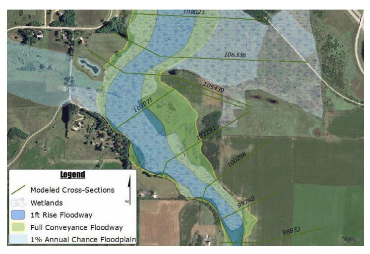
This map shows how an effective flow path or full-conveyance floodway can differ from a floodway based on a typical flood insurance study's 1-foot rise standard. Map created by ASFPM.
