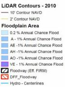
This image shows the traditional floodway delineation with black hatching and the larger extent of the DFF floodway in red., Only areas of shallow depth are excluded from the floodway permit requirements (e.g., areas above the 104-foot contour line).
