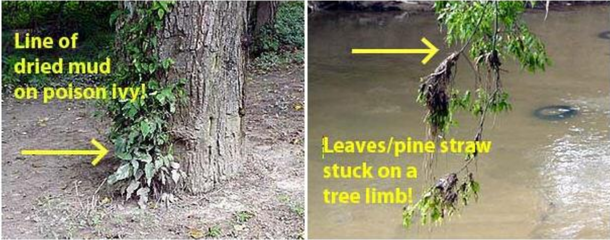
Figure 5- HWM from dried mud and debris. Courtesy of Georgia Water Science Center
